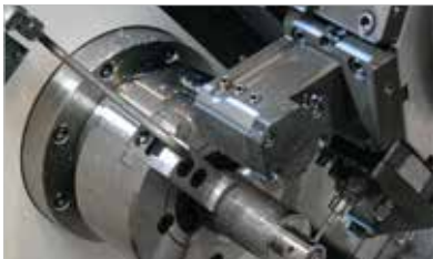
Chuck Air Blow (Upper Chuck)
