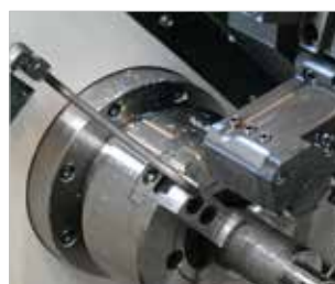
Chuck Air Blow (Upper Chuck)
